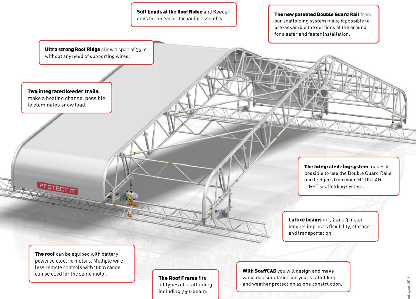
**Soft bends at the Roof Ridge** and Keeder ends for an easier tarpaulin assembly.
